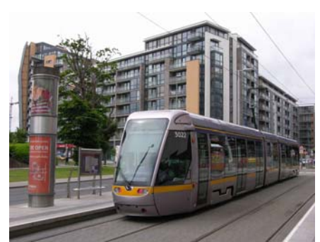
A low-floor LRT in Dublin shows how low-floor LRT would operate in Edmonton. Trains would operate on separate track space and stations could be integrated with sidewalks.
