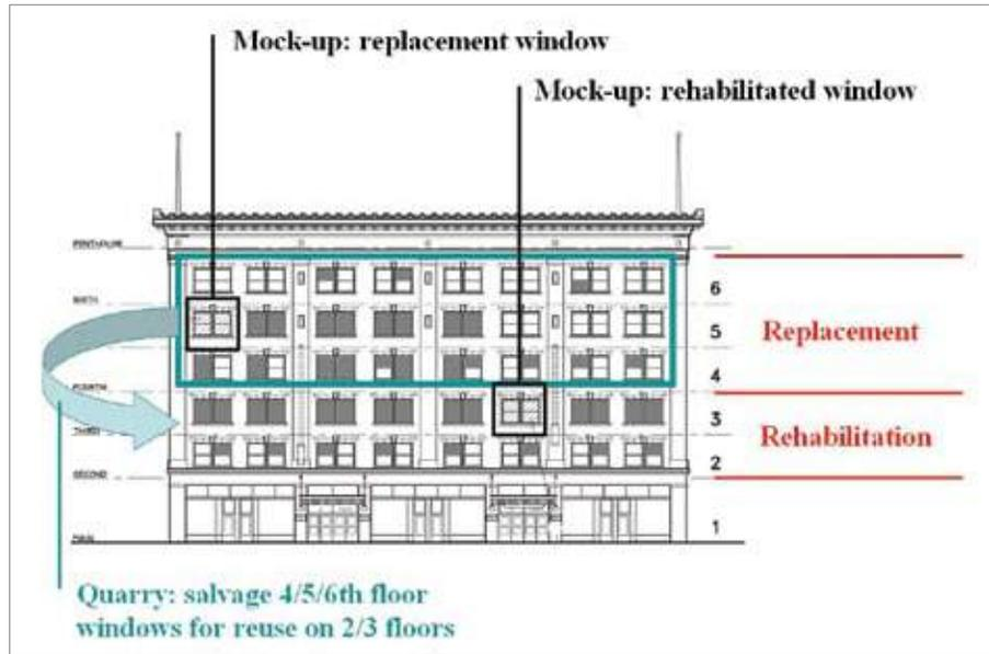
While rehabilitating the Lougheed Building in Calgary, the windows in the best condition were repaired and consolidated on the lower levels where they were most visible from the street. New windows based on the existing were specially constructed for the upper levels. The location and reuse of the windows was carefully and clearly documented both for construction purposes and for future reference.
