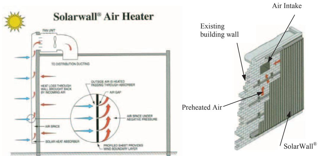
Figure 4: How a solar air heater works
