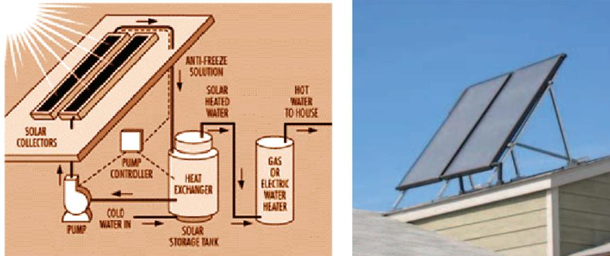
Figure 3: Solar hot water schematic<sup>17</sup> (left), and actual photo of system in Wha Ti, NWT (right)
