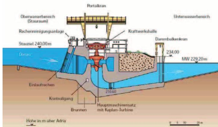
Figure 9: Schematic of low head hydro generator<sup>26</sup>
