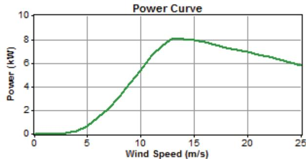
**Figure 14: Sample small wind turbine power curve**
