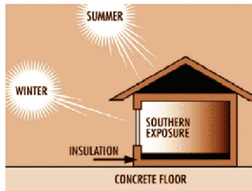
Figure 2: Diagram of how passive solar heating works in a home<sup>13</sup>
