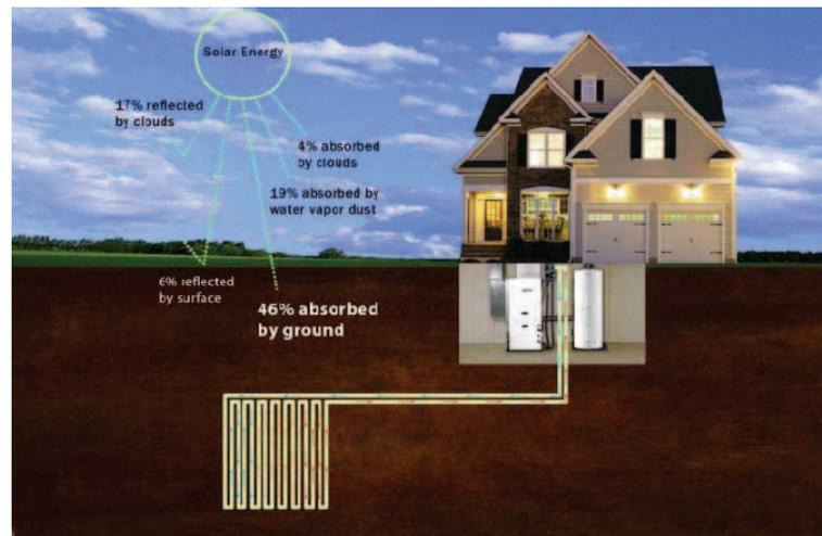
Figure 6: Ground source heat pump diagram (Picture credit: CleanEnergy Developments)
