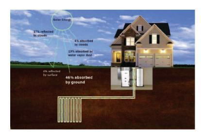
Figure 6: Ground source heat pump diagram (Picture credit: CleanEnergy Developments)
