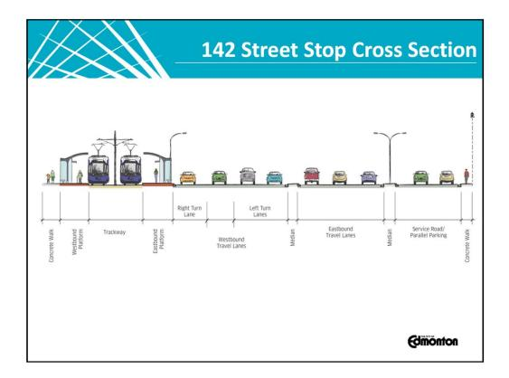
This is the cross section identified as 'J' on the last slide. This shows the relationship of the LRT with the stop, adjacent traffic and pedestrian areas.
