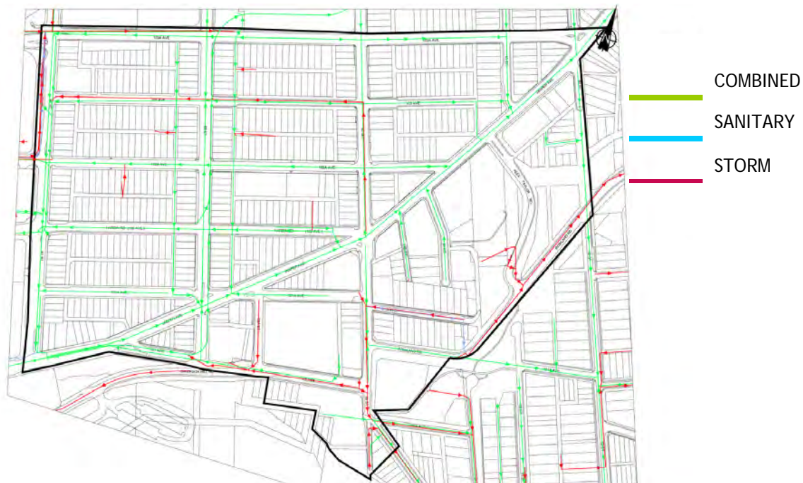
Figure 11 - Existing Lateral Sewer System
