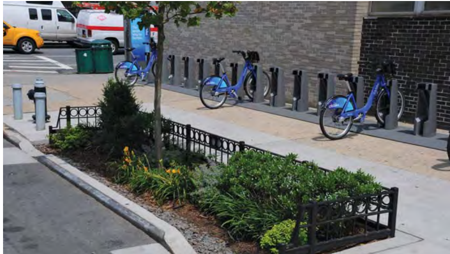
Bioswales beautify the streetscape in summer, could provide snow-storage areas in winter, and support healthier waterways year-round ▲
