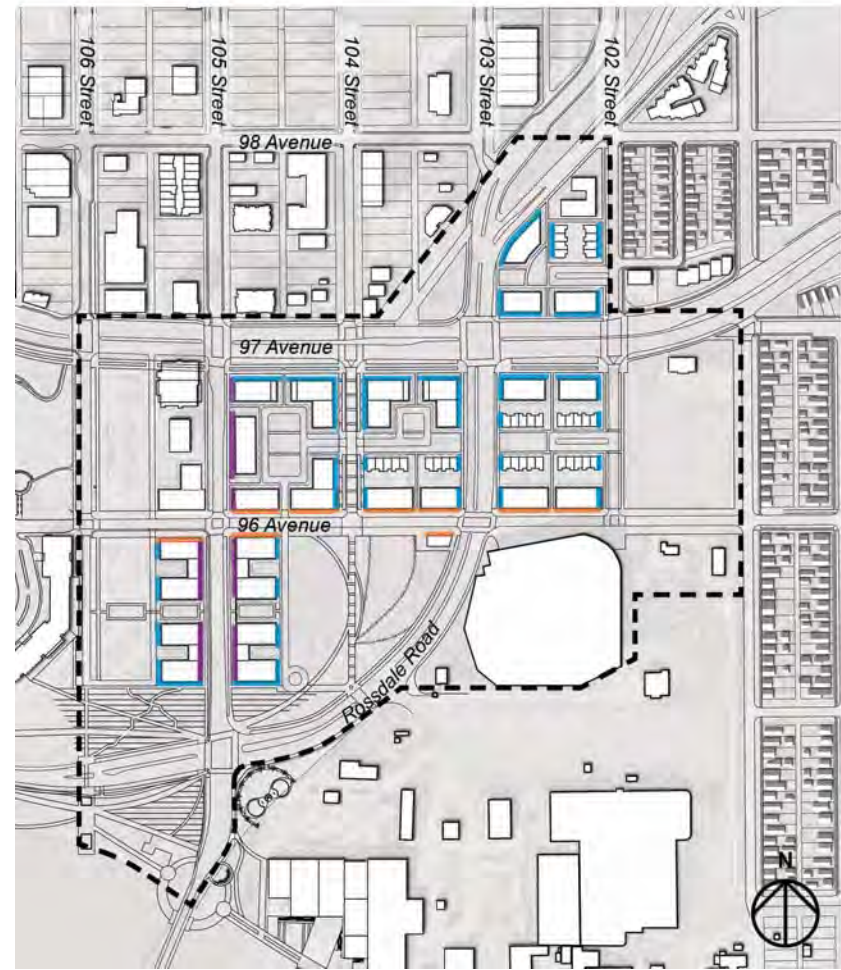
Figure 18 - Minimum Front Building Face Setbacks
