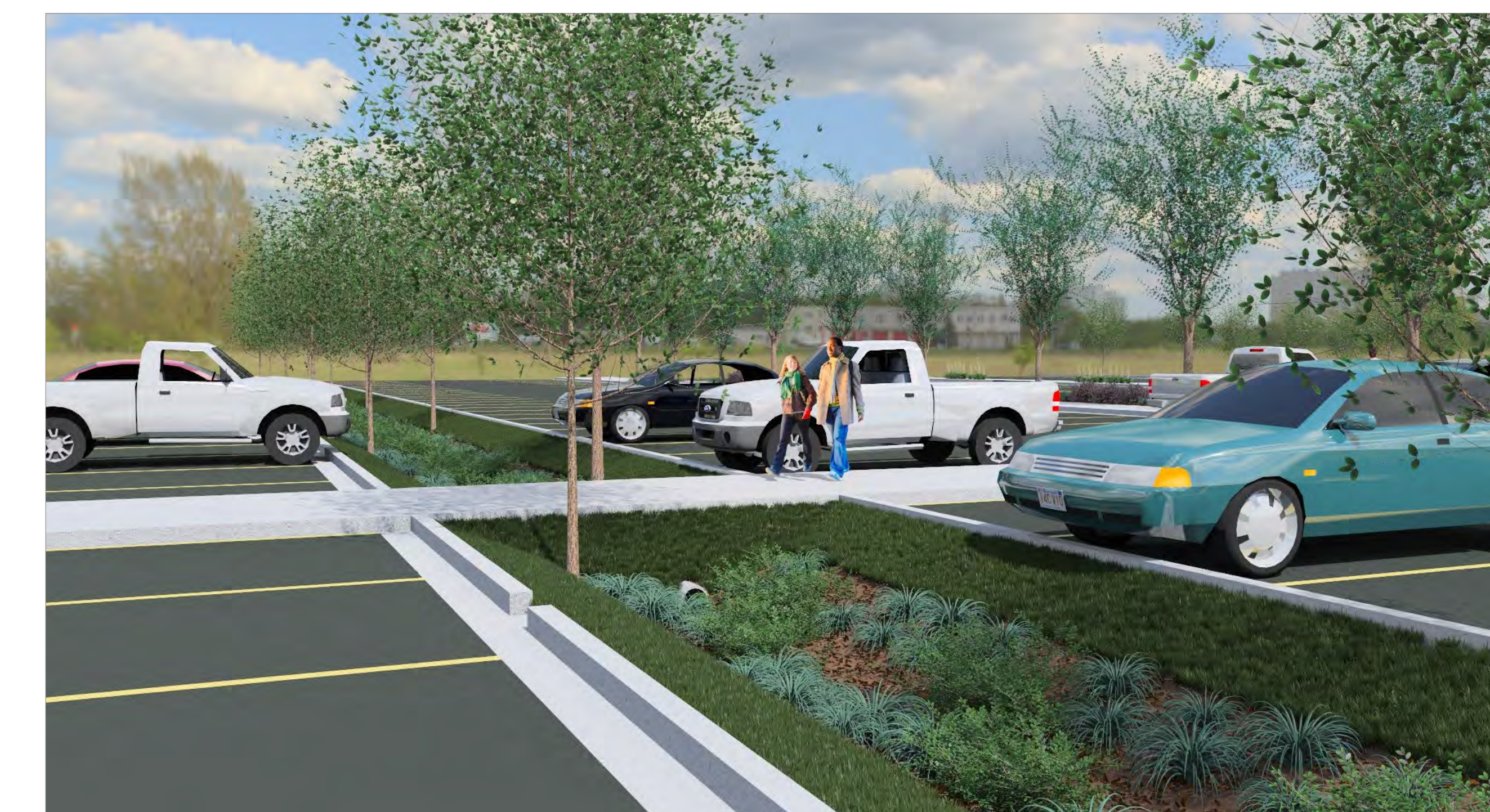
The existing drainage ditch (left) will be replaced with bioswales in the parking lot similar to the example rendering on the right, together with an underground drainage system
