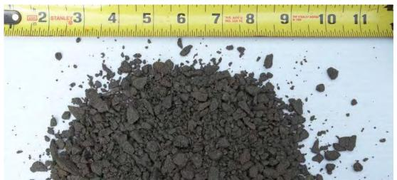
Fig.31: Fine Gravel (10minus) for looping pathway (shown at half-scale)
