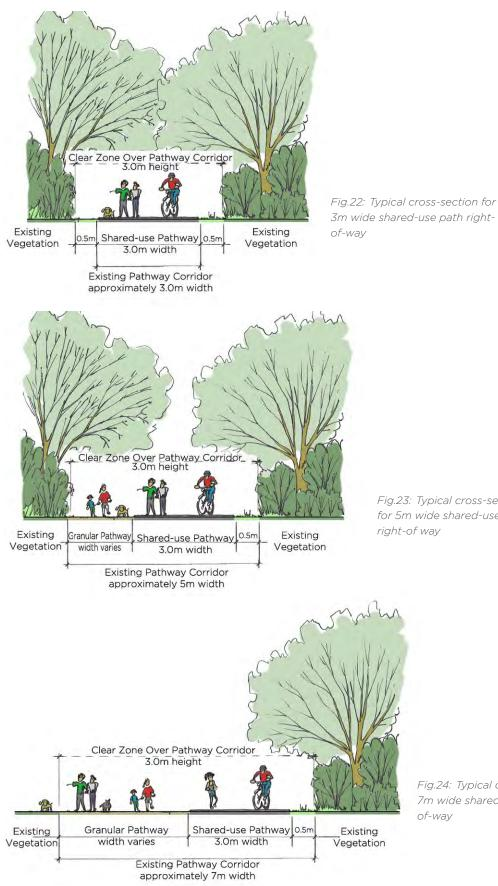
Fig.23: Typical cross-section for 5m wide shared-use path
