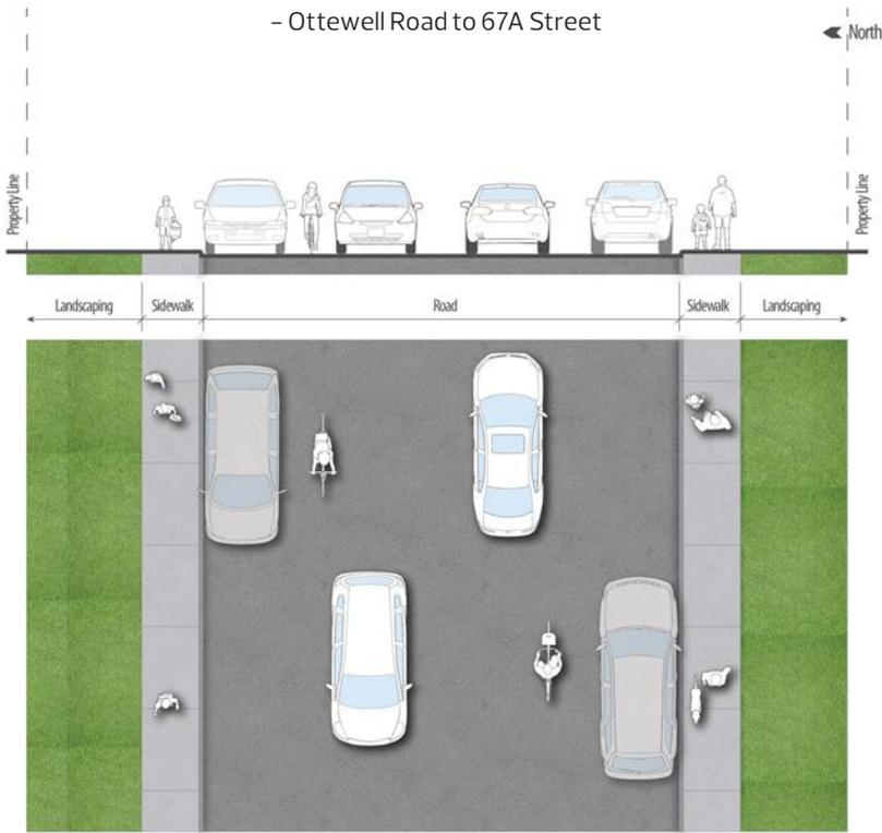
Figure 41: Cross Section | Proposed 93A Avenue
