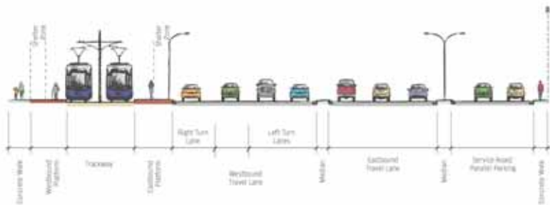
Cross-section A (Looking East) Note: Cross-section to be confirmed through Preliminary Design
