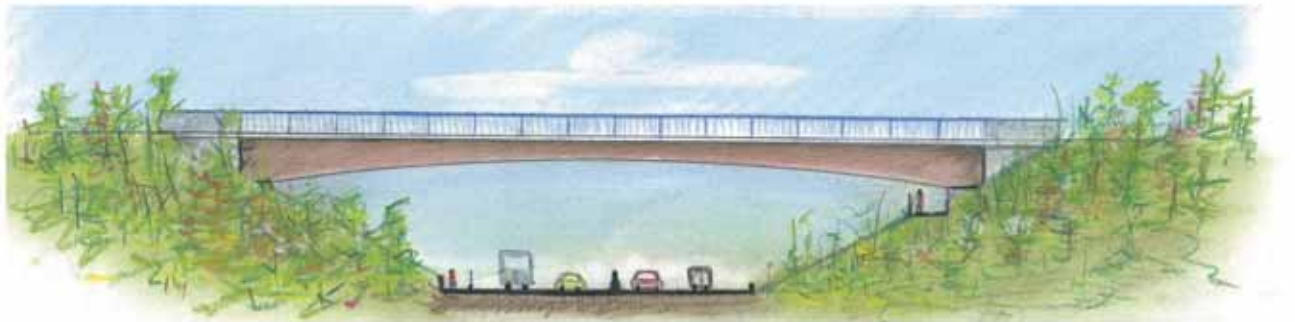
Single span girder bridge
