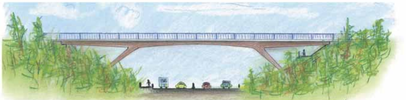
Rigid frame bridge
