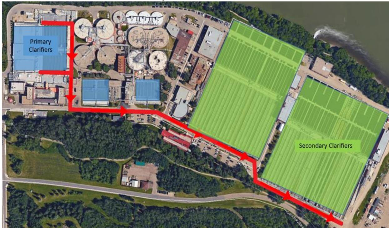
10. The red line shows the flow of the primary effluent, moving from the primary clarifiers on the west side of the plant (left hand side of the figure) along the south side of the plant, through the bypass chamber (just north-west of the red building), and on to the bioreactors in the east side of the plant (right hand side of the figure) for secondary treatment.
