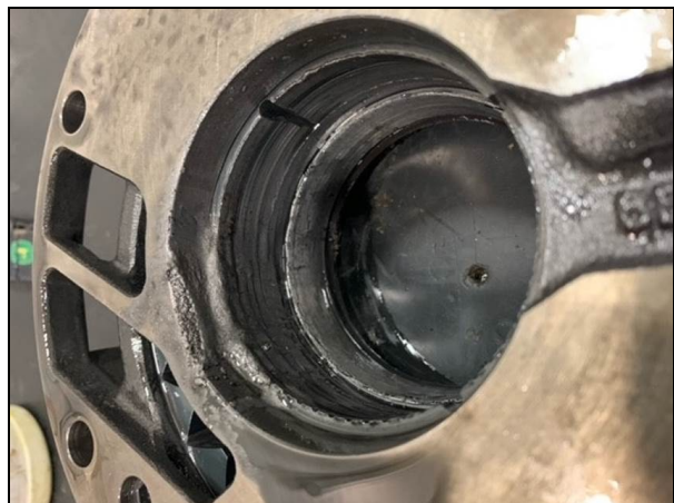
Figure 4: Damage inside the transmission oil pump.
