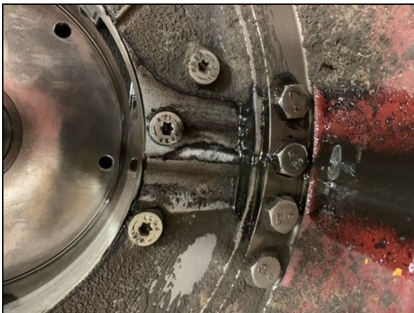
Figure 3: Metal contamination inside the transmission.
