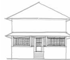
Typical window arrangement - Enclosed verandah
