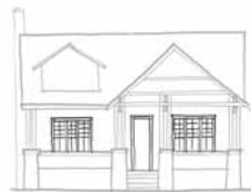
Typical window arrangement - Tri-partite windows
