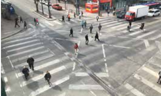
Pedestrian scrambles are one of the ways crossings can be made safer through design. In 2021, two additional pedestrian scrambles were installed in Edmonton, both in high activity locations along Whyte Avenue.
