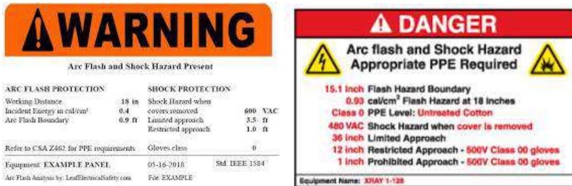
Figure 1 – Examples of Arc Flash &amp; Shock Hazard Labels
