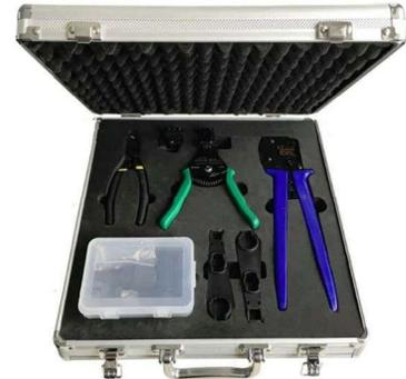
**Figure 4 – Quick Connect Assembly Tool Kit**
