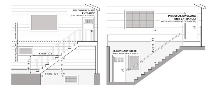
If there is not a second 'means of egress' other than by a single exterior exit door, then that door must be protected from all windows of the other dwelling and common spaces located within 3m (10') horizontally of the exit door(s) in facing walls or walls built at angles < 135°. This also applies to windows in exterior doors (see figure on the right; NBC(AE):B:9.9.4.6.)
