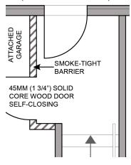
A Secondary Suite's only means of egress may not be through an attached garage. The access and exit from each dwelling may not be through the other dwelling, an attached garage or through a service room. All essential functions of a suite must be accessible from within the suite itself, and not through the main dwelling or common areas. Ensure that
