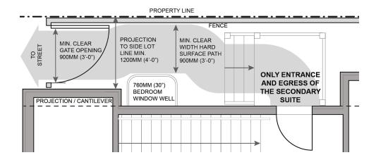
A suite exterior exit doorway, passageway and stair (or ramp) exposed to a window or hazard from the common area or another suite in a house with a secondary suite will need to be protected if there is not an alternate means of egress from the suite. Specifics are discussed here:
