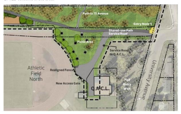
To address the safety concerns and make the entire area more functional as park space, a key upgrade proposed for this area involves removing multiple fences and gates and installing new chain
