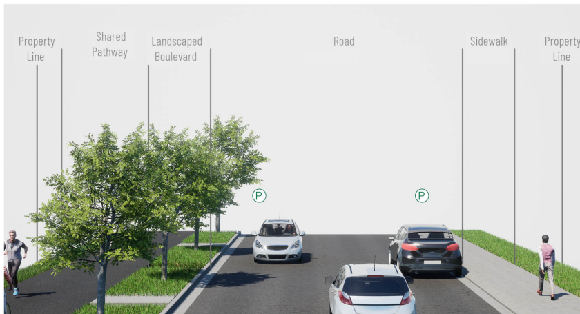
Scenario D: Shared pathway with landscape boulevard on one side of the road and a sidewalk without a boulevard on the other side. Parking unchanged.
