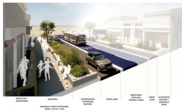
Whyte Ave – Bioswale and Rain Garden Example
