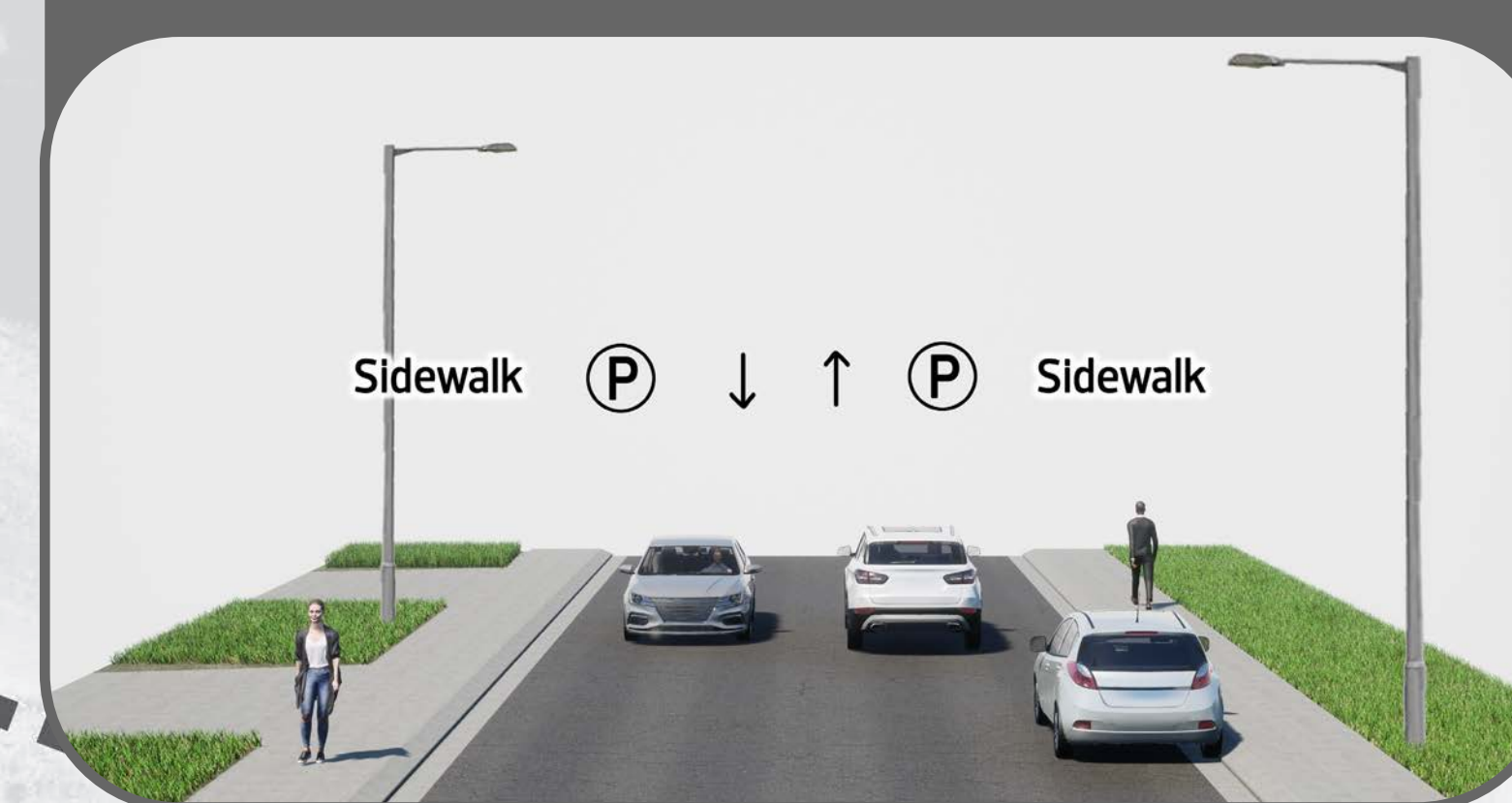
Typical local road with sidewalks next to curb
