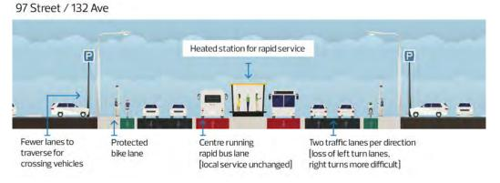
In Option 2 we see the bus lanes are centralized with a heated shelter in the middle. This option also hosts two vehicle lanes in each direction, plus the addition of a dedicated bike lane in both directions.
