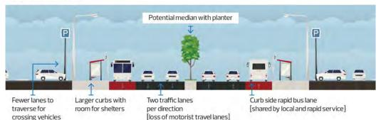
In Option 1 there are larger curbs with room for shelters, the addition of a bus lane means each direction of traffic is reduced to two lanes.
