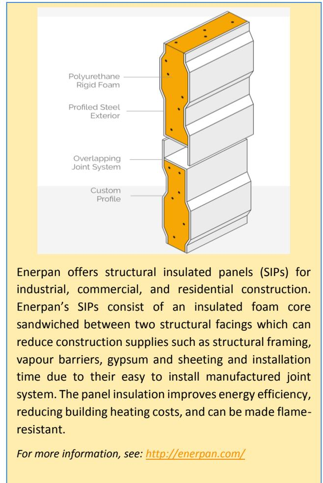
Enerpan offers structural insulated panels (SIPs) for industrial, commercial, and residential construction. Enerpan's SIPs consist of an insulated foam core sandwiched between two structural facings which can reduce construction supplies such as structural framing, vapour barriers, gypsum and sheeting and installation time due to their easy to install manufactured joint system. The panel insulation improves energy efficiency, reducing building heating costs, and can be made flame-resistant.
