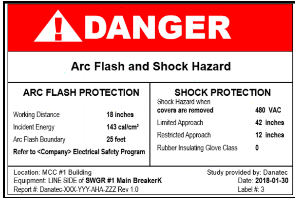
Figure H-3 – Detailed Arc Flash & Shock Danger Label for MCC/SWGR and other distribution equipment where Incident Energy is above 40 cal/cm 2
