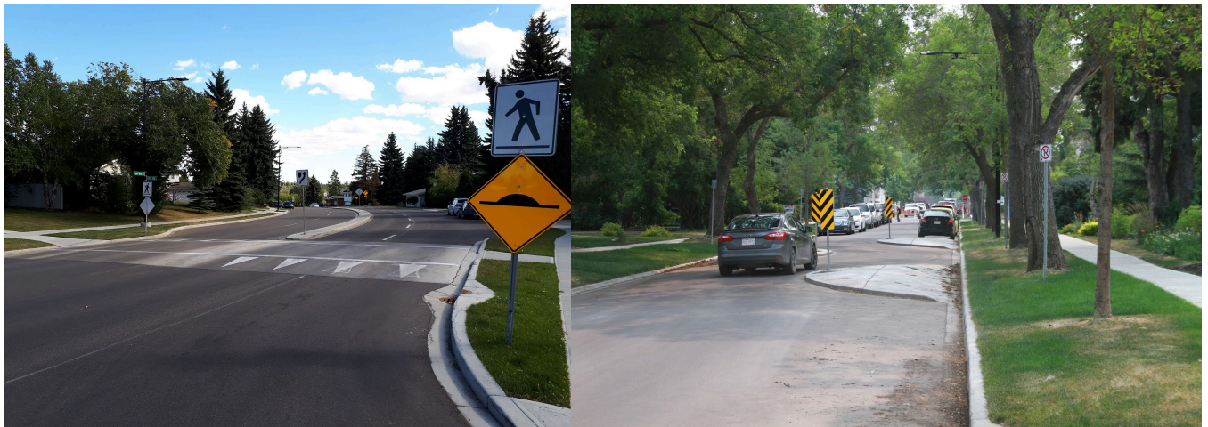
Figure 9 - A raised crosswalk, which is an example of a vertical deflection ( left image ). Chicanes, which are an example of a horizontal deflection ( right image ).
