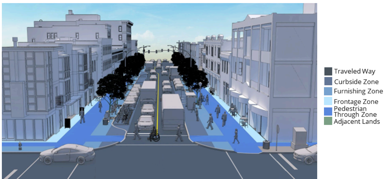
Figure 2 - This picture shows the zones for a street oriented commercial road.
