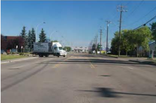
Figure 3.22C: Two-way or shared left-turn centre lane (Typically used in industrial area arterial streets)
