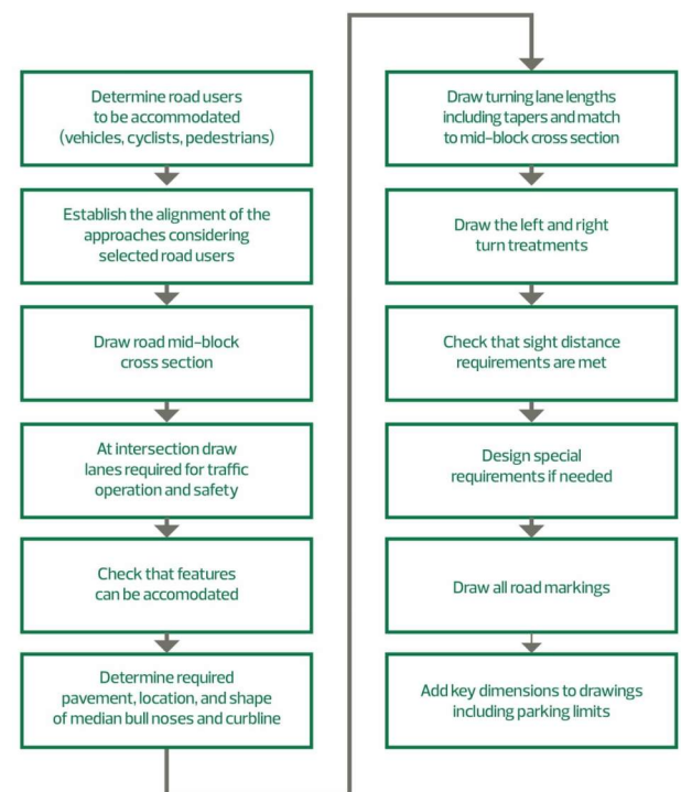
Figure 3.43 Intersection Design Process Flow Chart
