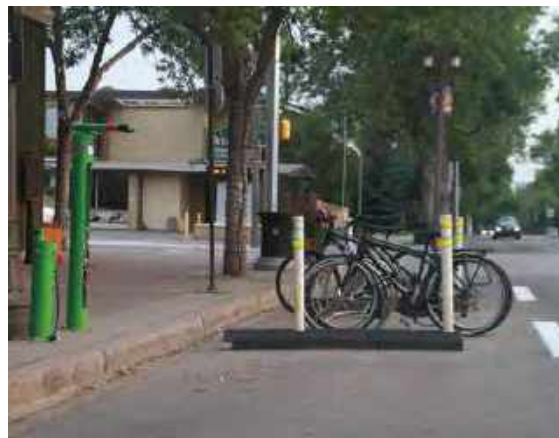
Figure 3.35 Bicycle Parking Corral in Ancillary Zone
