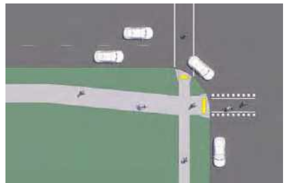
Figure 3.64 Intersection Shared-Use Paths Crossing (Bend-Out)
