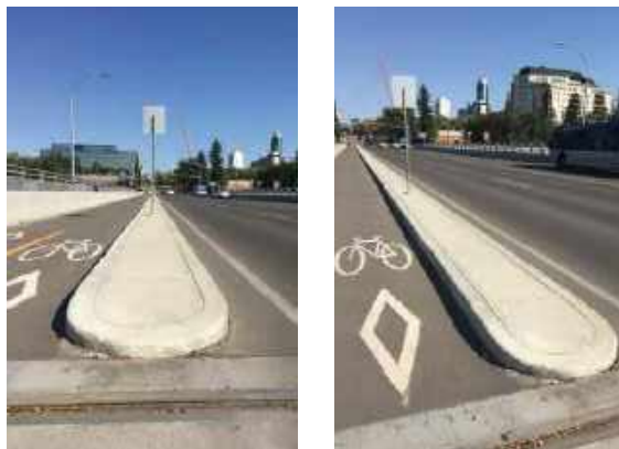
Figure 3.14 Protected Bike Lane Delineators
