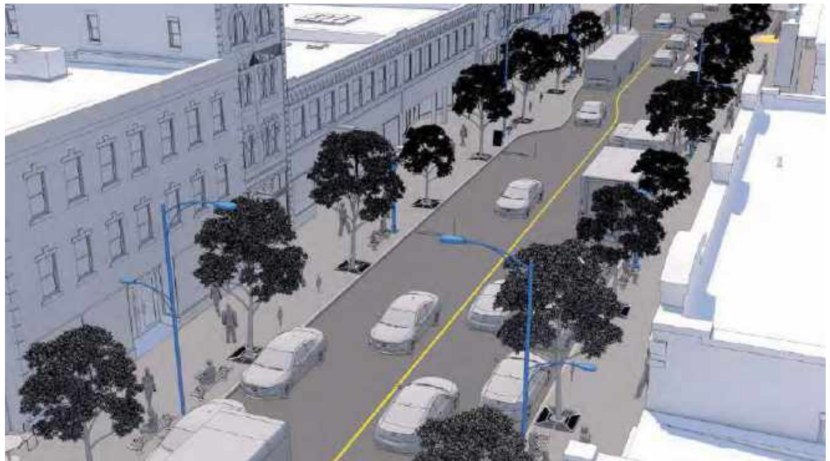
Figure 3.38 Street & Pedestrian Lighting Spacing
