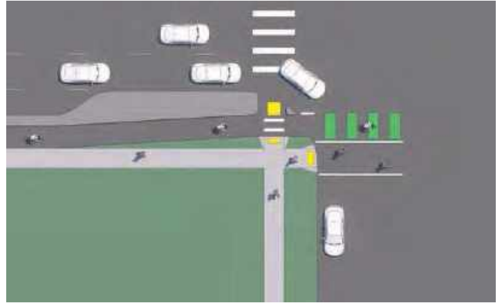
Figure 3.56: Protected Bicycle Signal Phase with Bend-In
