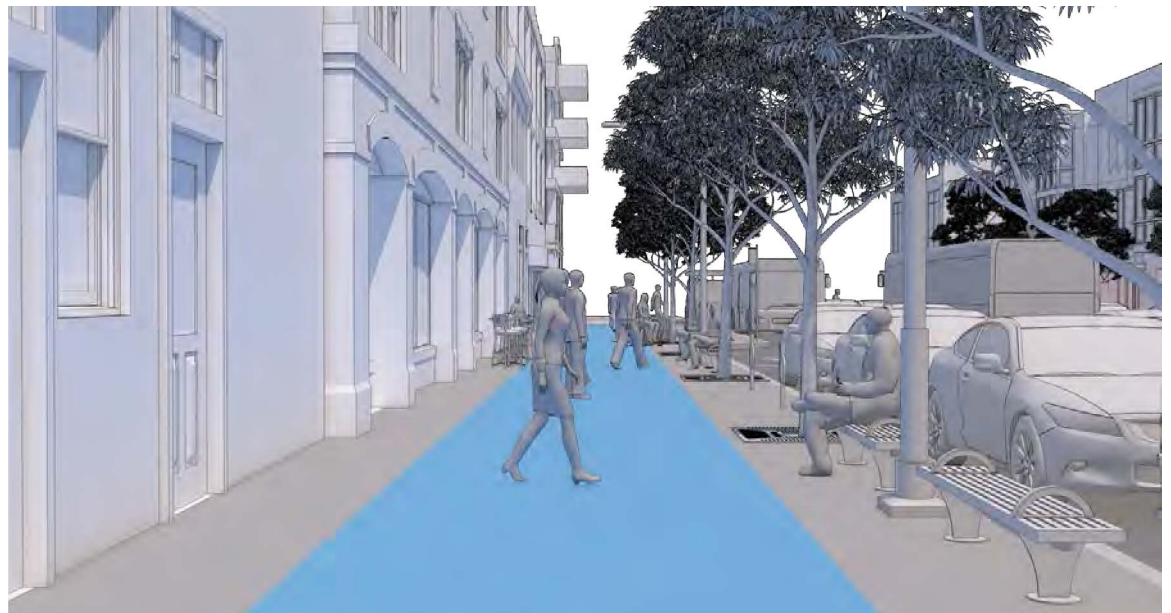
Figure 3.39 Pedestrian Through Zone
