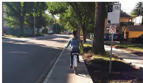
Figure 3.12 Unidirectional (Raised) Protected Bike Lane
