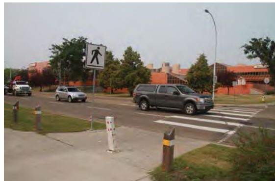
Figure 3.73: Typical Crosswalk Pavement Markings
