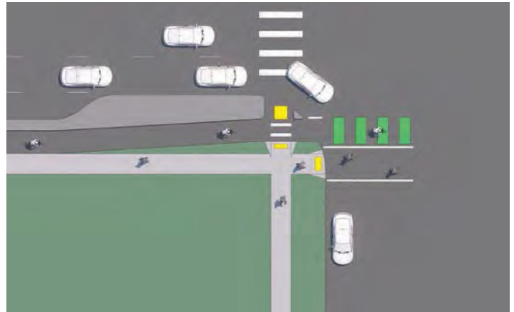
Figure 3.56: Protected Bicycle Signal Phase with Bend-In
