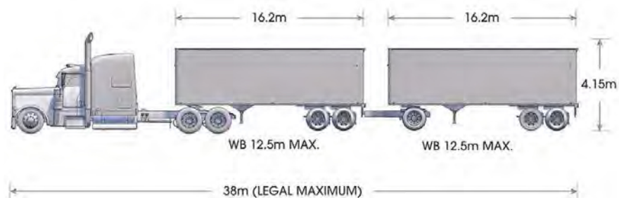
Figure 3.10 WB-21 Tractor Semi-Trailer Dimensions
