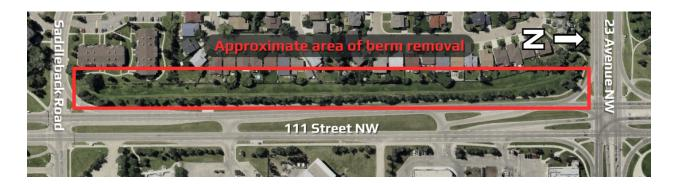
During berm removal, the top layer of soil will be removed using heavy machinery. The area will then be levelled to accommodate the LRT trackbed and an entrance for the LRT underpass at 23 Avenue and 111 Street. Efforts will be made to minimize noise, vibration and dust. Mitigation measures will be implemented to monitor and reduce these impacts. Once project construction is complete, trees and native vegetation will be planted along the alignment as part of the final landscaping plan.
