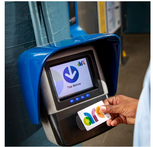
Arc fare validator at an LRT station
