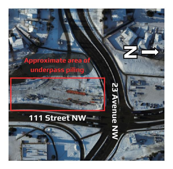
Large equipment used for the piling work will include drilling rigs, a crane and numerous trucks. The rigs will drill holes along the site of the future LRT underpass. These will then be filled with concrete that will eventually support the underpass. We anticipate the loudest work will occur during concrete pours. We thank residents and business owners along the alignment for their patience as we complete this important work.
